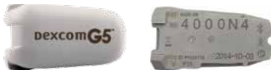
Figure 2. Dexcom G5 Transmitter Front and Back
