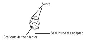
The adapter connects the cartridge to the infusion set. It has two seals to keep water from getting into the cartridge compartment. Two vents on the adapter allow air pressure to equalize. The adapter will not work properly if the vents are plugged, dirty, or if the seals are worn or missing.
